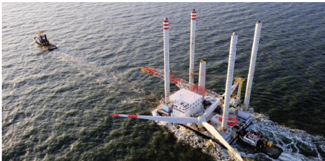
Figure A8-2: First turbine being transported to Alpha Ventus - July 2009. (Copyright: ©DOTI 2009)
